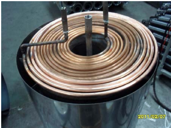
Fig. 3 Picture of heat exchanger coil located in the upper part
