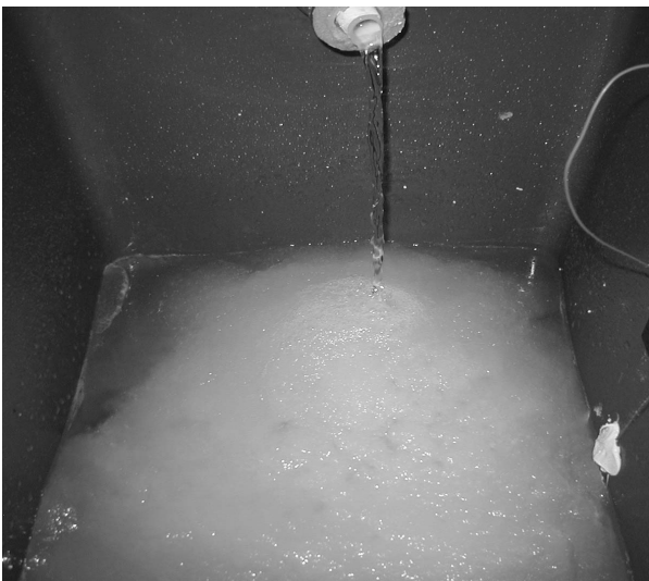
Fig. 3 The photograph of making ice slurry in slurry tank ( G_s=4 LPM, T_{b,i}=-5^{\circ}\text{C} )
