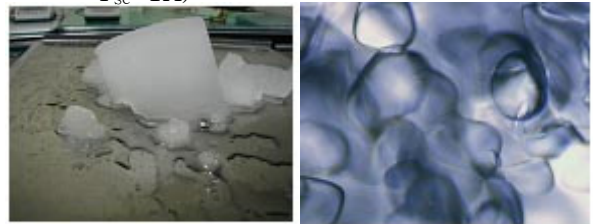
Fig. 6 Snapshot of Ice slurry and its particles (Sea Water 98 mass%, PG 2 mass%, \Delta T_{sc}=1\text{K} )
