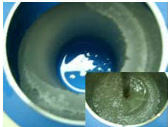
Fig. 9 Adhesion of ice on cooling wall (Lactic acid 7wt%)
