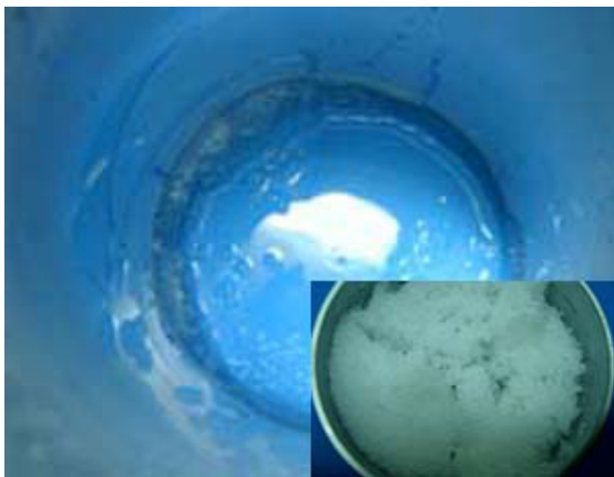
Fig. 5 Non-adhesion of ice on cooling wall (EG 4wt%, PG 1.5wt%, 1,6 Hexanediol 1.5wt%)
