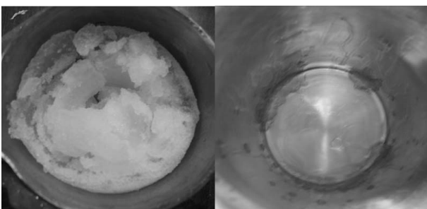
Fig. 6 Non-adhesion of ice on cooling wall (inside wall and bottom, EG 4wt% SCA 3wt% \Delta T_{sc}=4K T_{brine}=-7.5^{\circ}C )
