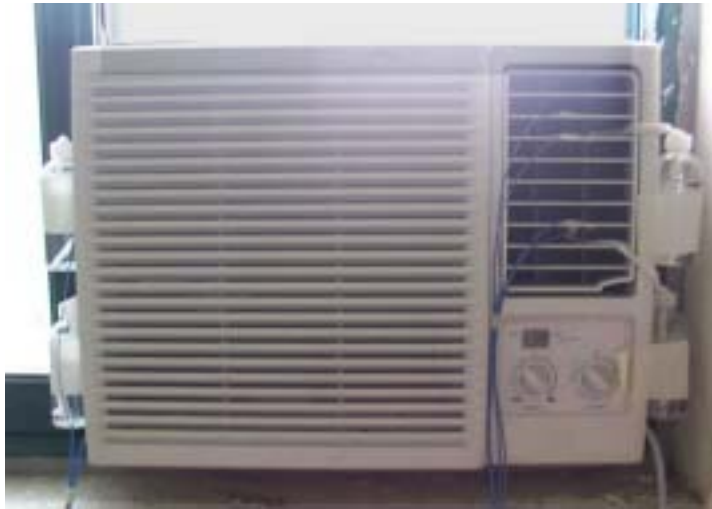
Fig. 10 Mesurment of dry and wet bulb temperature for air conditioner input and output
